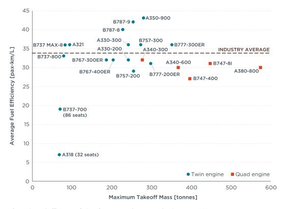
Figure 2. Fuel efficiency of aircraft types used on transatlantic routes, 2017.
